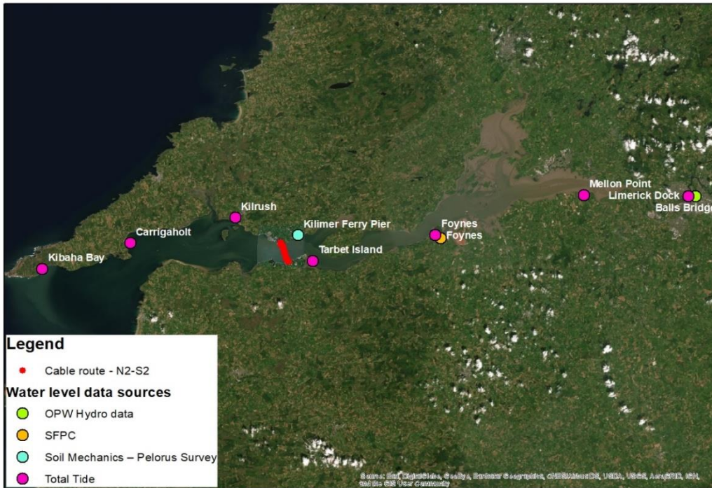
Figure 3.2: Location of the water level data available in the Shannon Estuary. This includes measures and predicted datasets.
